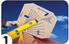
To determine roof pitch, place gauge on peak of roof as shown. Position straight edge as shown. Read roof pitch from printed gauge parallel to bottom of straight edge.
