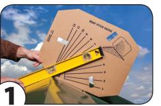
To determine roof pitch, place gauge on peak of roof as shown. Position straight edge as shown. Read roof pitch from printed gauge parallel to bottom of straight edge.
